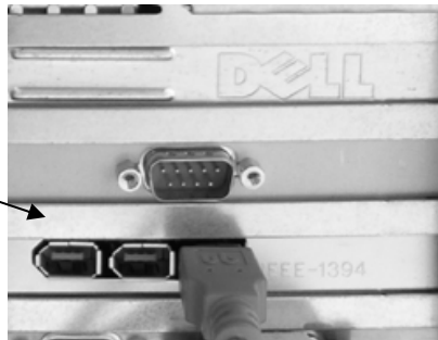
Firewire ports located on the back of the computer
